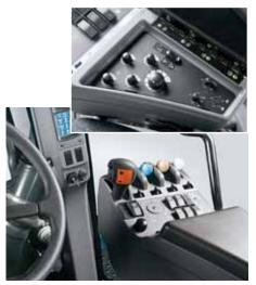
Right at hand ... controls for AutoShift<sup>TM</sup> hydraulic remotes, flow and timer, diff lock, hitch, custom headland management, optional slip limit, throttle and gear selection are integrated into the armrest for ready, comfortable access.
